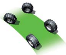
FRONT WHEEL STEERING MODE
