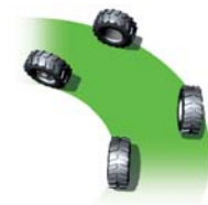
FOUR WHEEL COORDINATED STEERING
